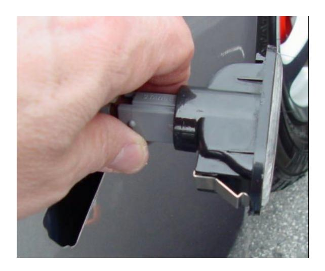
5. The marker is now ready to install. On one end of the marker you'll see a small black plastic slot/clip. At the other end you'll see a plastic clip. The black plastic slot mounts toward the front of the car. Slip the marker into place front first, with the notch in the plastic slot over the sheet metal. Then push it into place in the back (the plastic clip should snap into place, locking the marker into position). Do not force things, as the plastic clip is easy to break.
